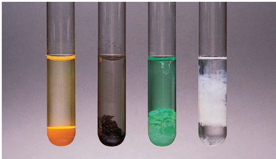
Figure 4.4 Appearance of several precipitates. From left to right: \text{CdS} , \text{PbS} , \text{Ni}(\text{OH})_2 , and \text{Al}(\text{OH})_3 .
