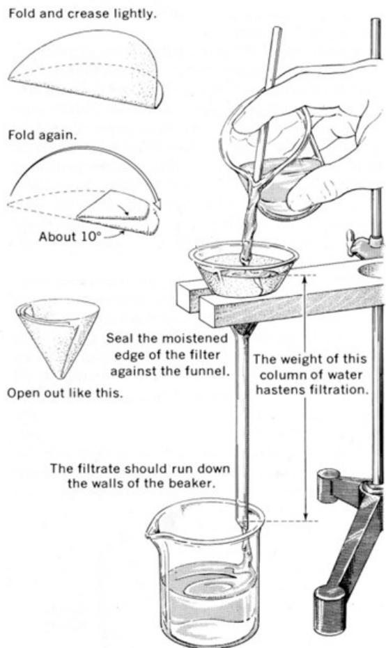
Fold a circle of filter paper in half and then fold again so that the edges do not meet but form an angle of about 10°. This will allow for a better fit to the funnel.
