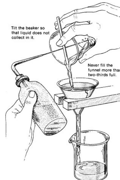
When filtering a precipitate, first decant most of the supernatant solution into the funnel. Then, using a wash bottle with distilled water flush any precipitate remaining in the beaker into the filter. During this process, the liquid level in the funnel should never be filled more than 2/3 full.
