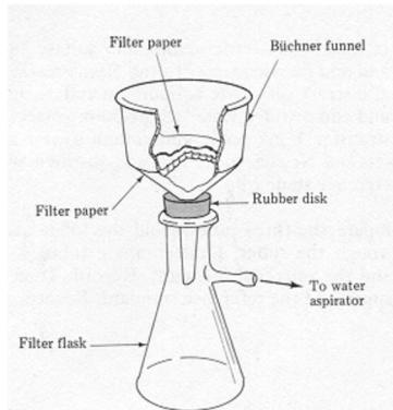
The flat filter paper and the vacuum make for speedy filtration.
