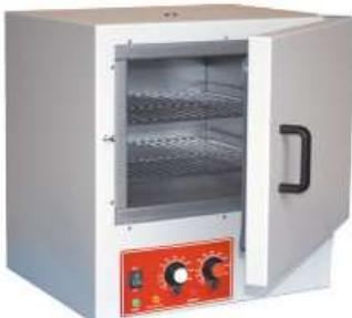
The filter paper and precipitate are then put in a drying oven which will heat the filter paper to evaporate the water. The oven must be warm enough to evaporate the water, but not so hot as to decompose the precipitate or burn the filter paper.
